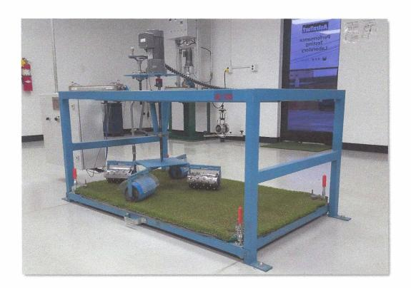
The material provided was subjected to artificial mechanical wear of a maximum duration of 5,000 cycles on the JE-108 wear tester. The sample was visually inspected and photographed, both initially, and after every 1000 cycles.
