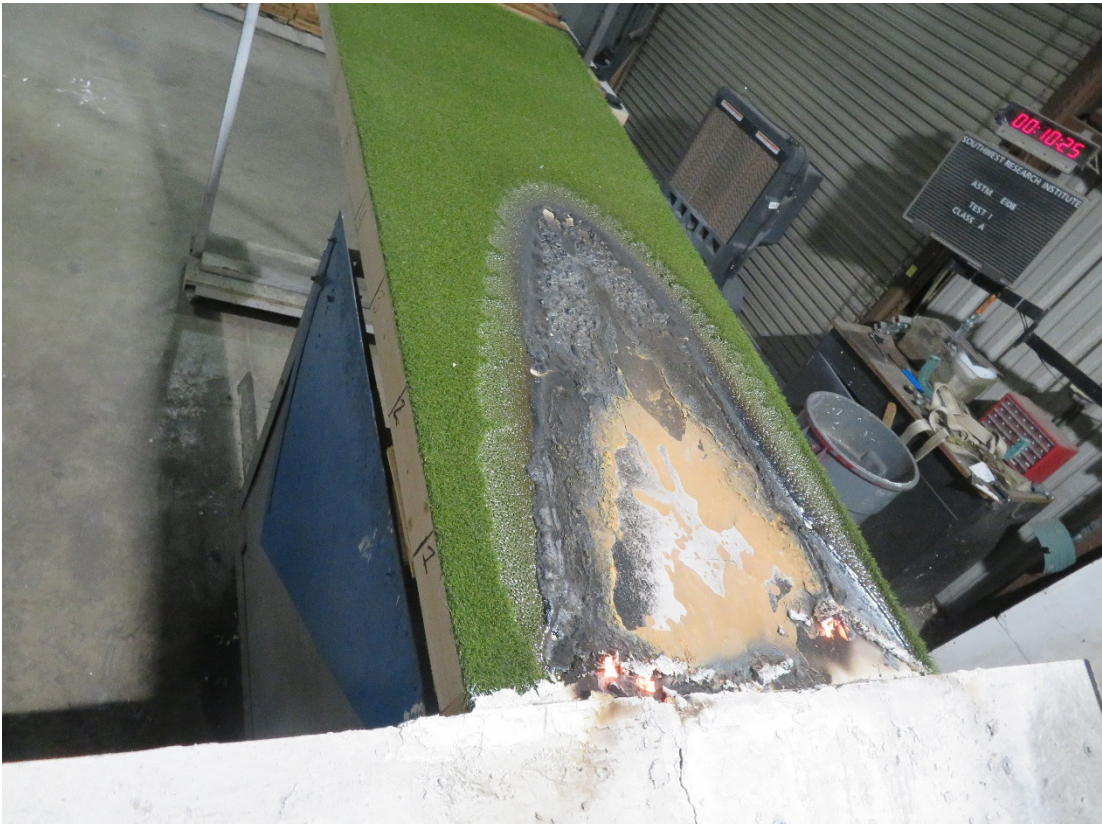
Figure B-4. Typical sample at the end of the SoF test.
