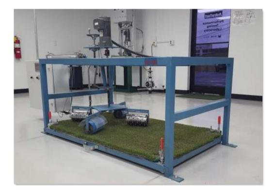
The material provided was subjected to artificial mechanical wear of a maximum duration of 2,500 cycles on the JE-108 wear tester. The sample was visually inspected and photographed, both initially, and after every 500 cycles.
